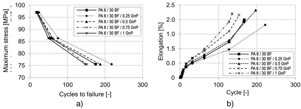
Figure 9. S-N curves and elongation of hybrid composites
