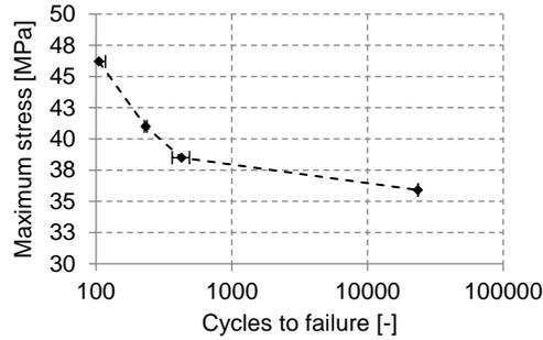
Figure 3. S-N curve for polyamide 6
